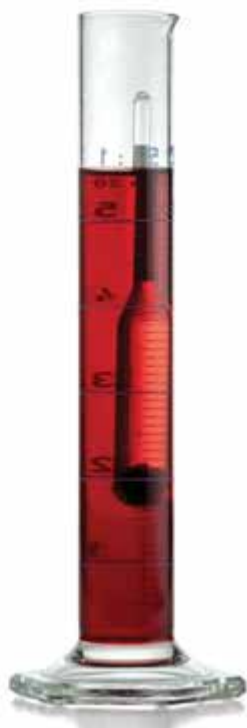
Measuring specific gravity with a hydrometer
